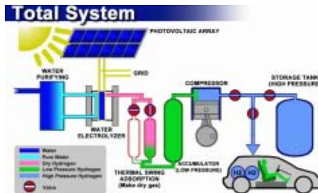
Figure 2: Schematic of Honda's hydrogen fueling station
