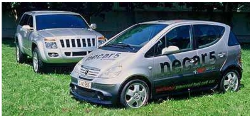
Figure 6. Two prototype automobiles powered by fuel cells, the NECAR 5 and JEEP Commander, from DaimlerChrysler (Photo courtesy of DaimlerChrysler).
