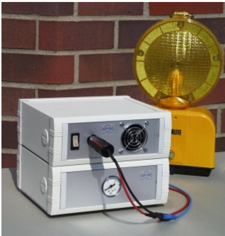
Figure 9. A prototype portable fuel cell provides 50 watts electrical power. The supply of hydrogen for this unit, by Heliocentris, is stored in the attached metal hydride canister.
