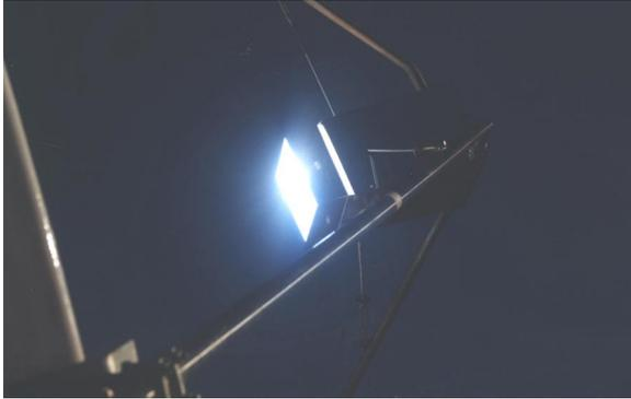
**Figure 7:** Photovoltaic receiver of Dish #2 while in operation. The incident power density is 25.3 W/cm<sup>2</sup> in average. One can notice the “flux modifier” in front of the solar cells.
