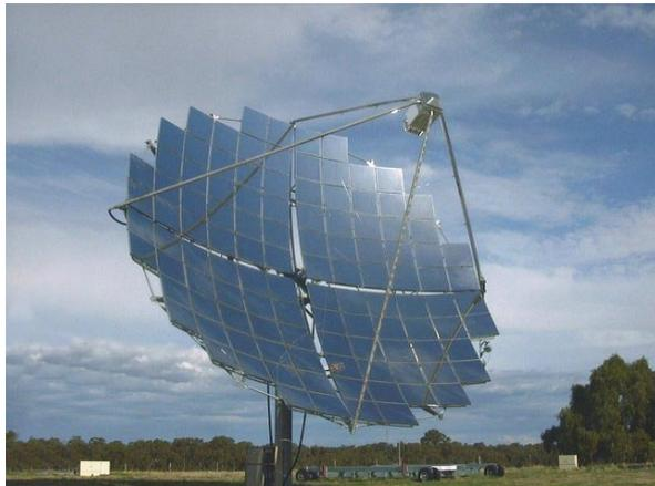
**Figure 8:** Solar Systems large-area (130 m<sup>2</sup>), high-efficiency concentrator PV system with 24 kW rated power.
