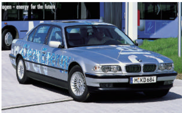
Figure 12: Vehicle with bivalent engine for hydrogen and gasoline fuels
